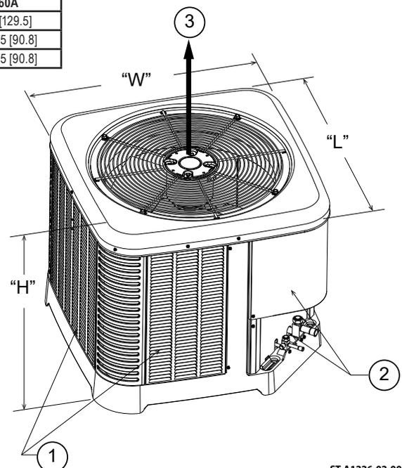
**Figure 1: Unit Dimensions & Clearances**
