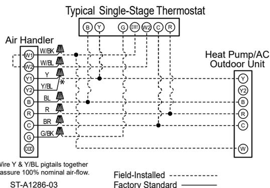
**Figure 25: Typical Single-Stage Thermostat: Heat Pump With Air-Handler**
