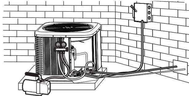
**Figure 20: Evacuate Air and Moisture from System**
