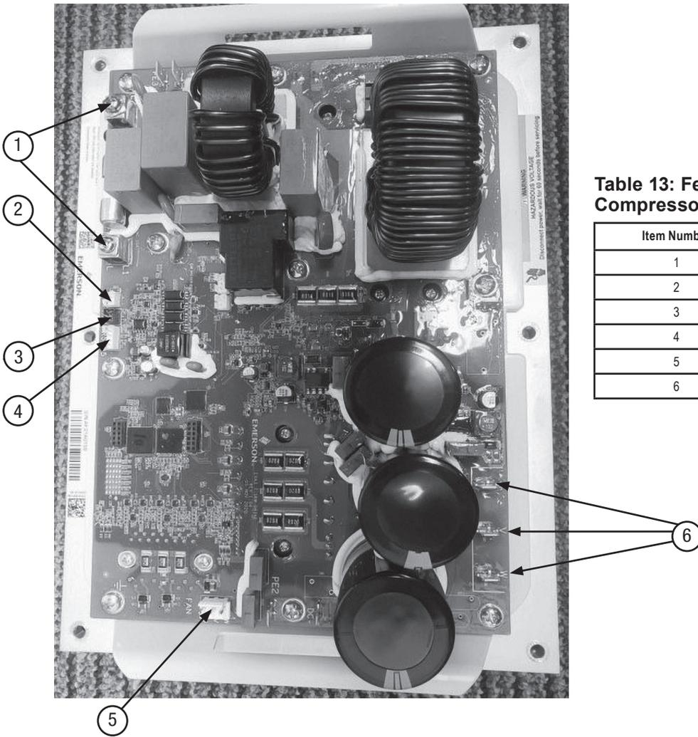
**Table 13: Features on the Power Inverter Compressor Control**
