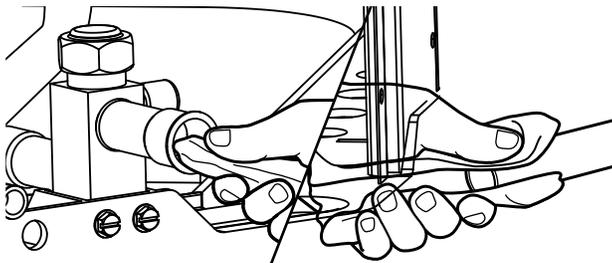
Figure 13: Clean Inside Fittings and Outside Tubing
