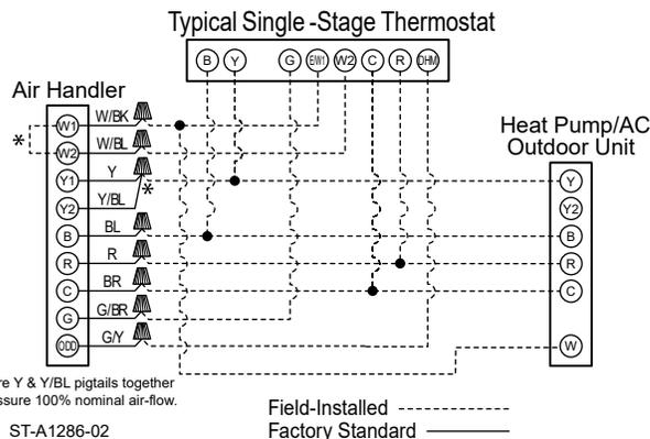
**Figure 24: Typical Single-Stage Thermostat: (-)P18AZ Heat Pump With Air-Handler Using A Thermostat With Dehumidification**
