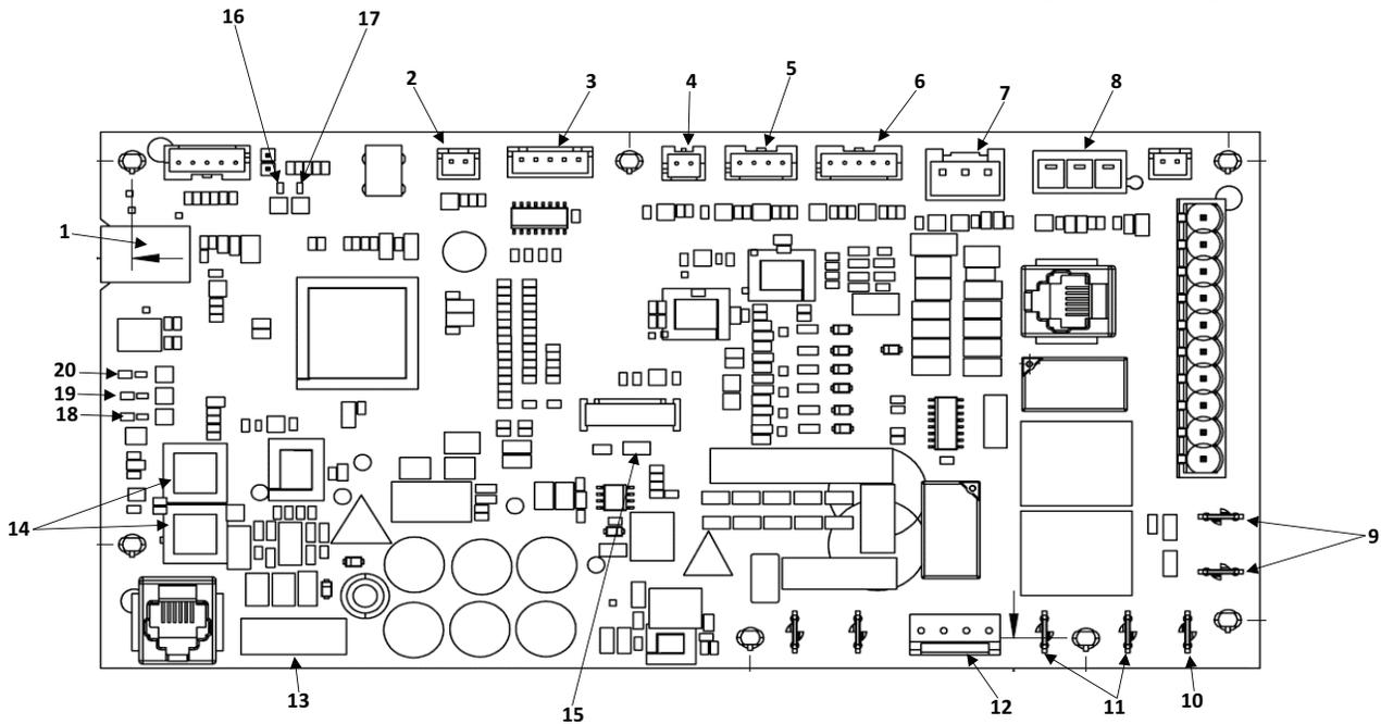
Figure 30: EcoNet™ Universal Outdoor Control (UODC) Connection Diagram
